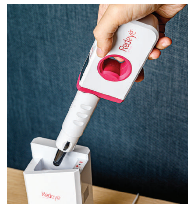
With optical sensing technology, users only need to put the handheld device in water. The device will indicate the current situation of fecal occult blood through a red or green colored indicator on the device.
