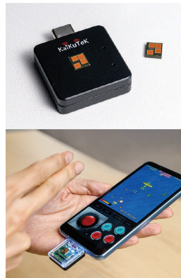
KaiKuTek's powerful integration skill spawned the world's first fully integrated embedded system that combines the 60GHz mmWave radar and dedicated AI accelerator.
